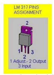
The transformer is the heart of the power source. Though of the same importance is LM317 integrated circuit. This IC can be obtain under two forms of packages: TO-3 and TO-220. Using the latter package, the mechanical work to mount it on the heatsink is much simpler.
