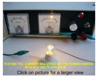
terminal posts of the source. Then, slowly turn the potentiometer to increase the voltage, watching at the same time the needle in the voltmeter. The filament bulb will start getting red and slowly reach its' full brilliance. Don't force this brilliancy or the bulb will pass away. At the same time check the needle of the ampmeter. Don't allow this needle to reach the right top portion on the meter face.
