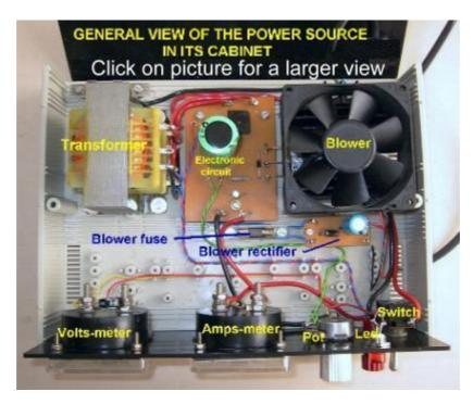
A regulated power source is not only an instrument that supplies direct current to your circuits at the desired level...it also allows you to have a previous idea about how the circuit operates. Having a volt-meter and an ampere-meter at the ouput of the unit, one knows immediately if there is a short or open circuit in the circuitry layout. And you would know first hand, if the current is excessive or too feble at the set-up voltage.
