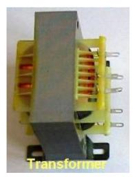
First, it is important to have a good transformer! That is, a transformer that does not get heated when the unit is working for a long time. My transformer has two entrance inputs; one 220 VAC and the other for 120 VAC. The transformer ouputs can deliver up to 3 amps, though I limit the power source only to 1.5 amps. The two outputs are 9 - 0 - 9 volts...allowing you to connect them in series to get 18 volts...or in paralell to get a stronger current. I used the '18 volt' connection.
